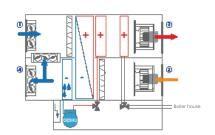
1 FRESH AIR 2 RETURN AIR 3 SUPPLY AIR 4 EXHAUST AIR
