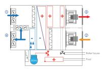
Dehumidification is ensured by the heat pump refrigeration cycle coupled with a heat pipe. Recovered heat is transferred to the supply air side, on the heat pipe and the aircooled condenser, in order to heat the dehumidified air.
